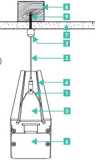
Installer must ensure that the slot orientation in ceiling barrel allows suspension wire to remain perpendicular at all times in all orientations
