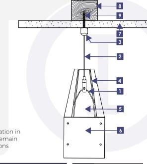
Installer must ensure that the slot orientation in ceiling barrel allows suspension wire to remain perpendicular at all times in all orientations
